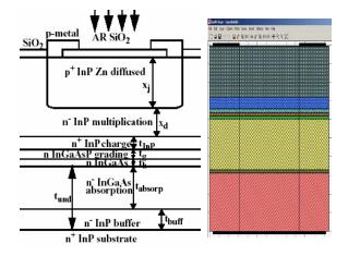
Optical absorption is mainly in InGaAs layer and impact ionization mainly in n- InP layer.
